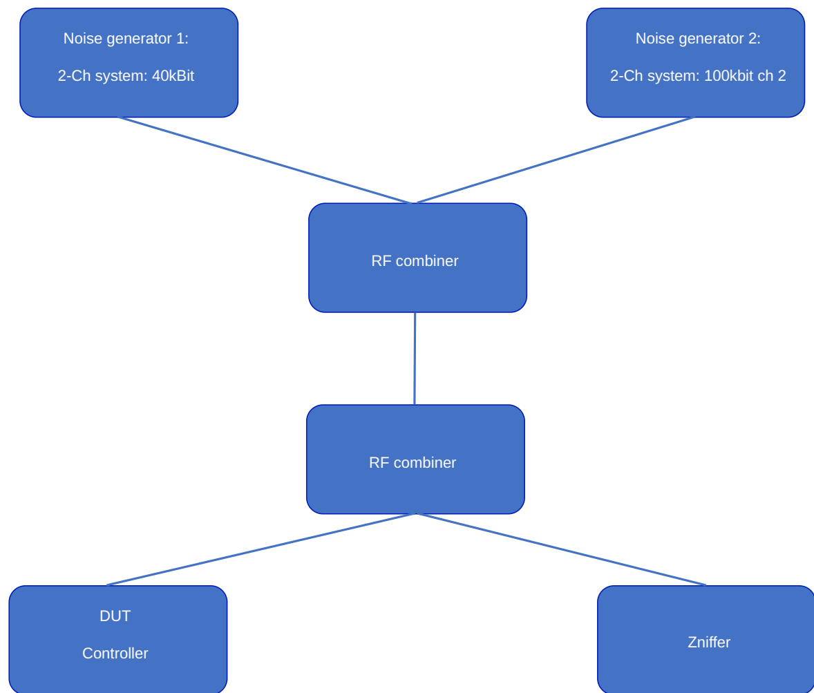
Figure 3.6: Connection structure for 2-ch frequencies
