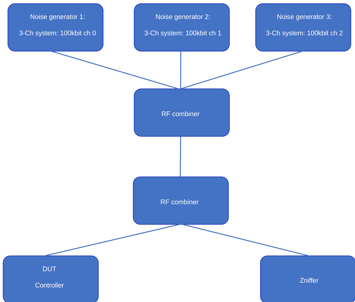
Figure 3.8: Connection structure for 3-ch frequencies
